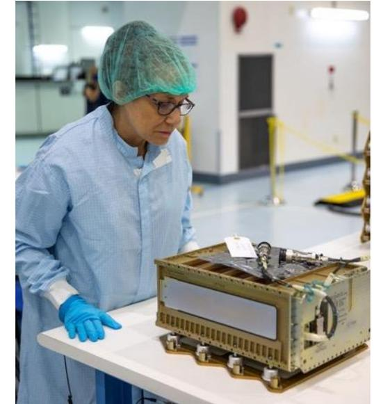
Use a miniature high-temperature Mid-Wave Infrared (MWIR) sensor to characterize the lunar surface.
